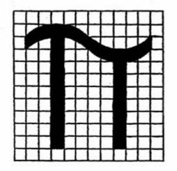
2. The minimum height of the Pi marking shall be 5 mm. For transportable pressure equipment with a diameter less than or equal to 140 mm the minimum height shall be 2,5 mm.
