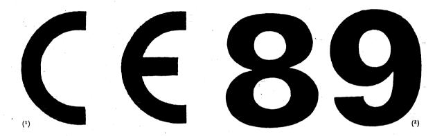
The vertical dimensions of the different components of the EC mark must be perceptibly the same and not less than 5 mm.
